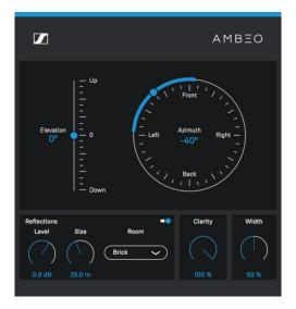
The AMBEO Binaural Panner allows engineers to position mono or stereo sources within a 3D soundfield and preserve the right balance between the tonal quality of the source and its 3D perception.
